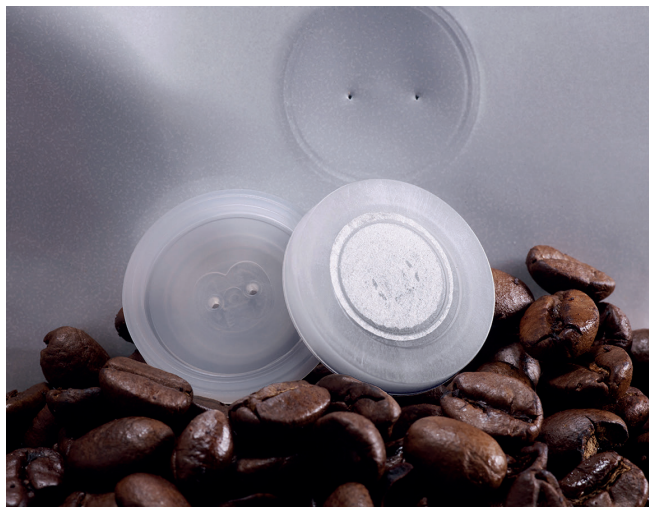
The Bosch VIS aroma protection valve is connected to the packaging film by ultrasonic welding. The valve enables degassing and at the same time prevents the inflow of harmful oxygen © Emerson
